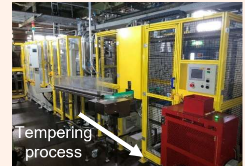
Dedicated quenching and tempering machine for CVJ outer races
