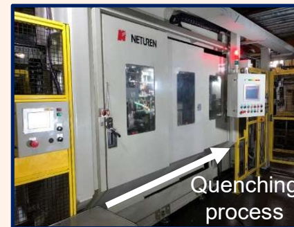
Dedicated quenching and tempering machine for CVJ outer races
